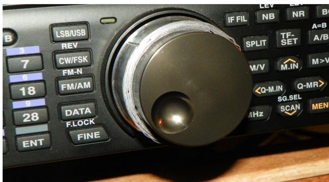
The photo above right shows the knob with one roll of tape wound and installed back on the rig. Not very pretty at this point. Which leads to one last minor task – cut the rubber ring in half and install on the modified knob. The effect is much better looking and keeps hands and fingers away from contact with the lead tape.
