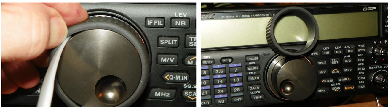
I inserted cable ties (serrated side up!) between the knob and the ring and was able to pull the ring off with a pair of forceps (or small needle nose pliers).
